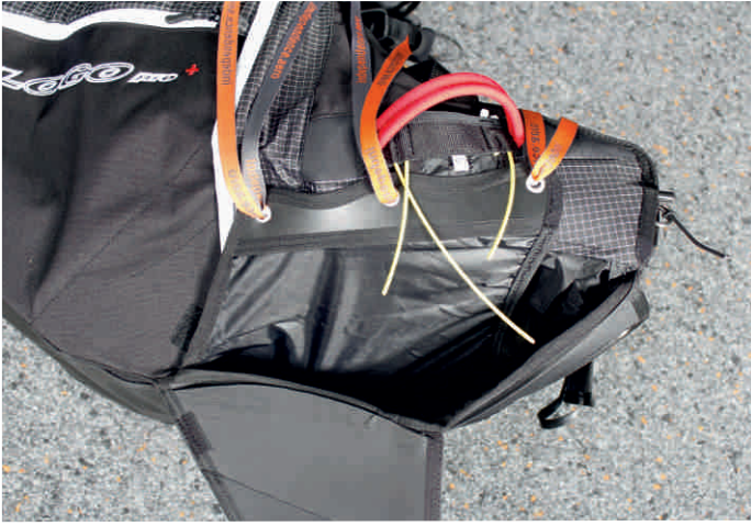
5. Close the tension band with the packing cords.
