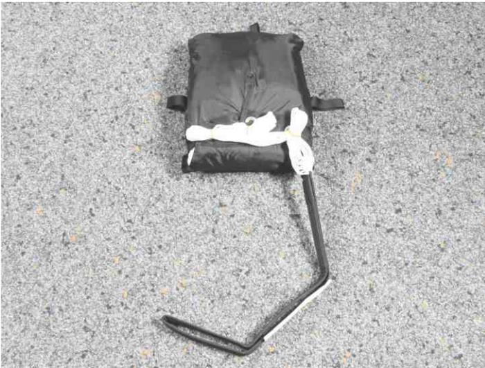
13. Close the container with the lines. First in the middle then the sides.
