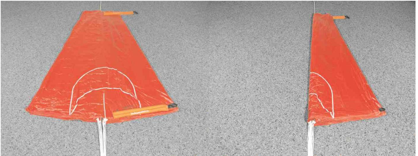
3. Lay all segments until segment 1 (stamped segment) is on the top, then put a weight (sand bag) on it.
