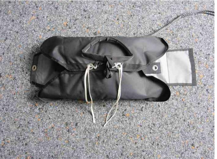
1. Stow the release handle at the loop in the middle of the deployment bag. Place the bridle at the side of the container which you prefer.
